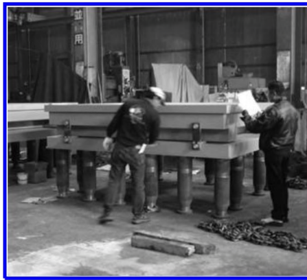
Figure 10. Giant shear keys with a design horizontal load of 31000 kN for the steel bridge near Taichung of the Taiwan High Speed Railway.
