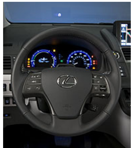
Figure 5 The steering column of the new Lexus HS 250h sedan is equipped with an infrared camera that reads your face while you drive—detecting whether you are watching the road.
